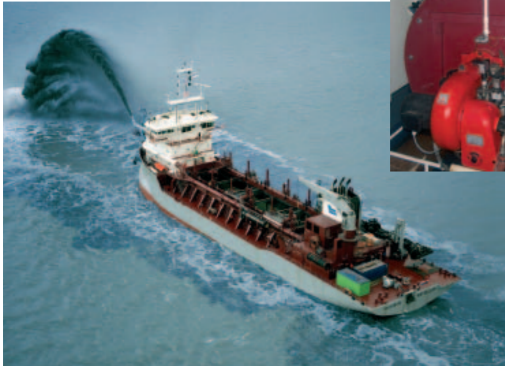
Hopper dredger, thermal oil heater with a capacity of 1.000kW and exhaust gas boiler with 860kW
