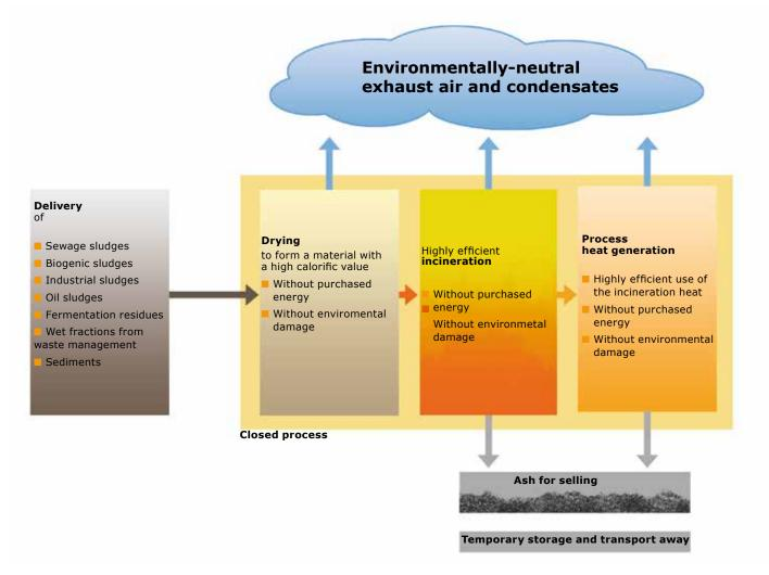
The greatest possible efficiency and economy are therefore achieved in the closed plant and process concept. However, thanks to the modular plant components, the concept is open to future changes based on new requirements.
